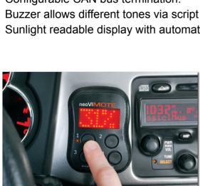
The light weight pendant can be mounted to the dashboard using Velcro ensuring easy reach for the driver.
