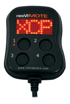
The scripting feature allows you to program the pendant to do complex message transmission and decoding for such protocols as XCP, GMLAN, ISO14229/UDS, and J1939.
